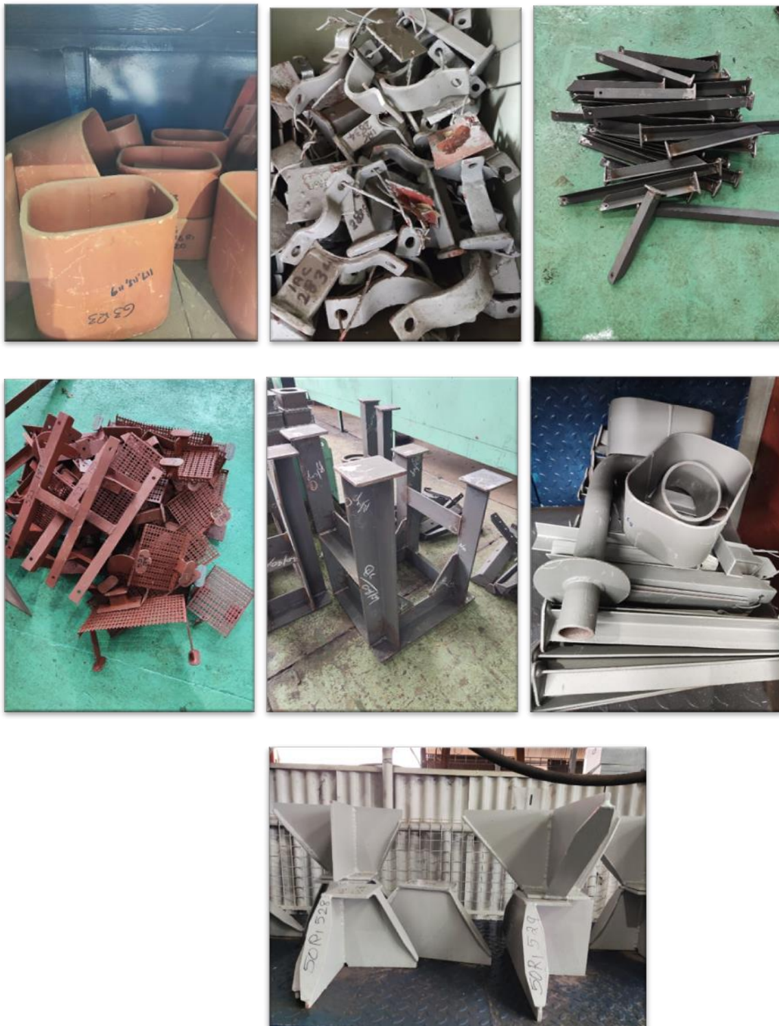
Fig 4. Fabrications done at Sheet Metal Shop (Coaming, pipe supports, cableway supports, equipment seats etc.)
