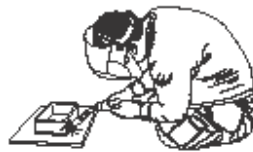
Horizontal MAG welding
