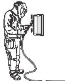
Vertical MAG welding
