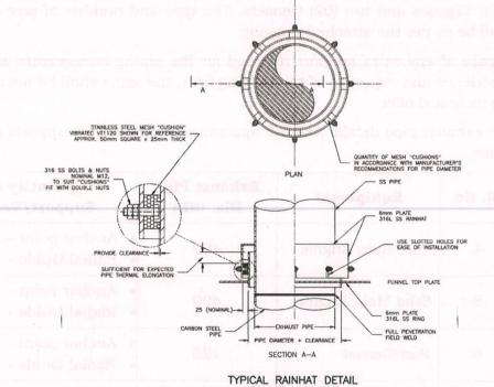
TYPICAL ONLY - NOT TO SCALE APPLY TO SPECIFIC PIPE SIZE AND INSTALLATION
