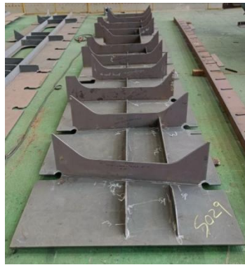
Fig. 11 Sub – Assembly after Web and Flange welding
