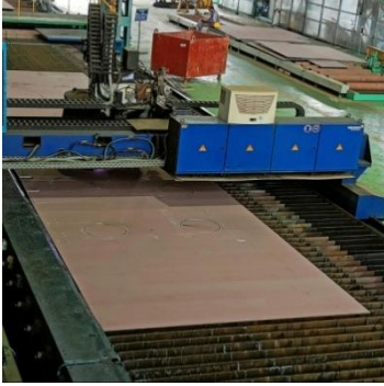
Fig. 1 CNC plasma cutting
