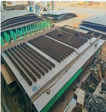
Fig. 13 Panel welding/ Stiffener Welding
