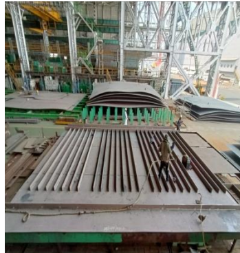
Fig. 14 Panel welding/ Stiffener Welding
