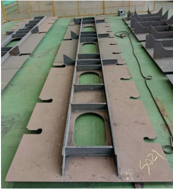
Fig. 10 Sub – Assembly after panel and stiffener welding.
