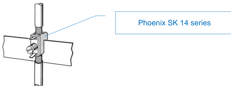
Figure 37 360-degree earthing is preferred.
