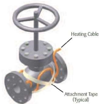
Heating Cable Serpentine on Valve
