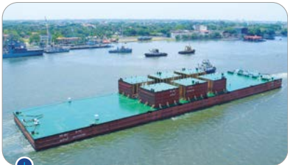
Deck Cargo/ Jacket Launch Barges
