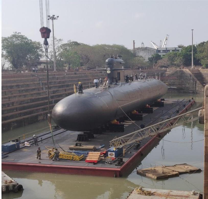
Separation of newly built submarine from Pontoon at Hughes Dock
