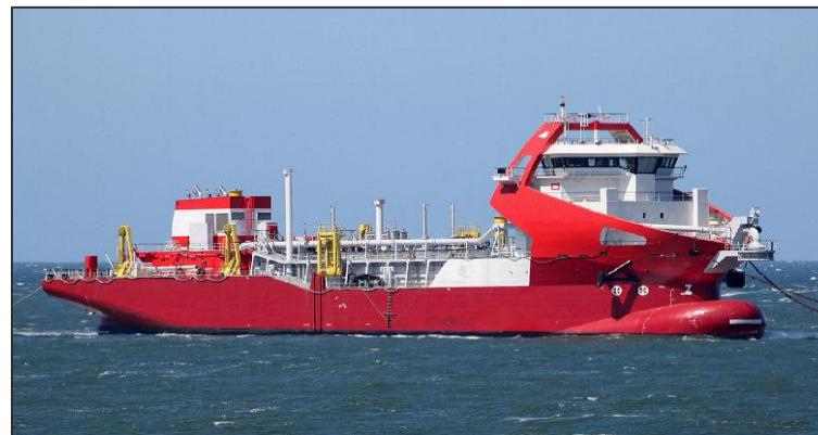
Hopper Suction Dredgers
