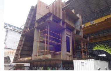
*Block fabrication of 1200 Pax cum 1000 Tonne Cargo vessels (2 nos) in advanced stages. Block erection to commence by Oct 2018.*
