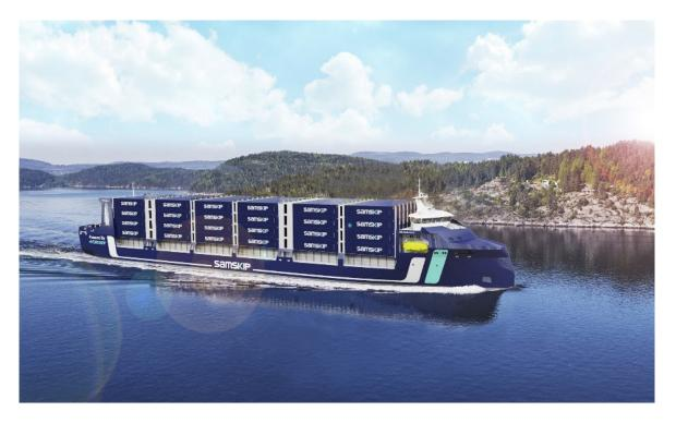
This SEA SHUTTLE project is one of the First Zero Emission Feeder Container Vessel in the World using Green Hydrogen as the fuel. This is an ambitious project admitted under the Norwegian Government green funding programme aimed at emission-free transport solutionsby adopting sustainable path breaking future technologies. In zero emission mode, each vessel is expected to achieve around 25,000 tons of  $CO_2$  reduction per year.
